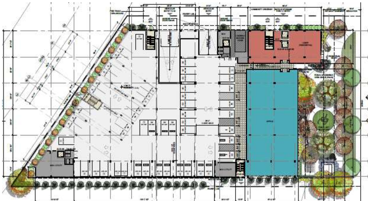
First floor layout with “full” commercial office space indicated in blue and some of the common space area in red.
