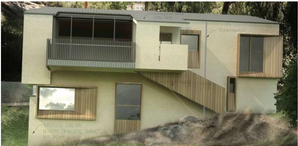
Previously submitted design for rear (East) façade showing wood material finishes and downspouts to water retention barrels.
