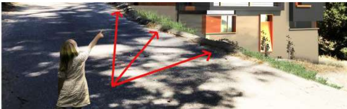
Low curb or berm to channel water away from site and prevent mud slides
