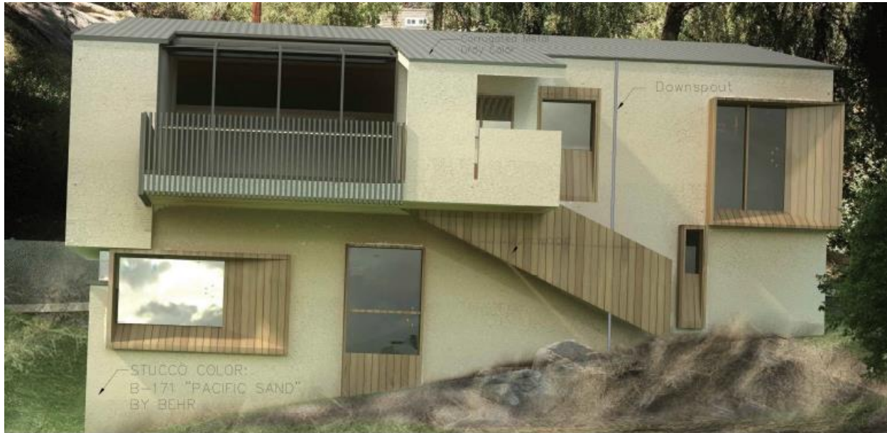
Updated rendering of rear (East) façade showing new balcony design, wood accents, new “Sand” coloration and downspouts to water retention barrels.
