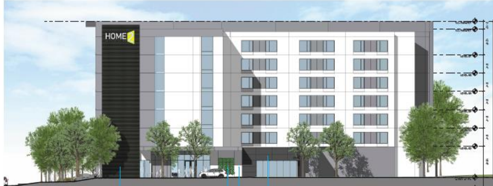
West façade showing main guest entry, porte cochere, and large dark grey ribbed metal architectural enhancement (left).
